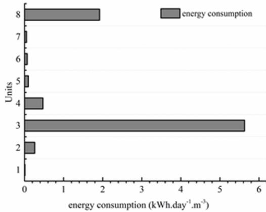
**Figure 2.** Electricity consumption of pumps and mixers
