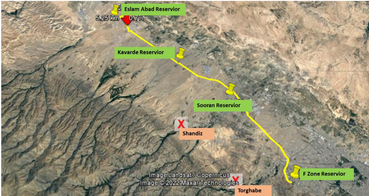
Figure 1. The approximate path of the water transmission line west of Mashhad.
