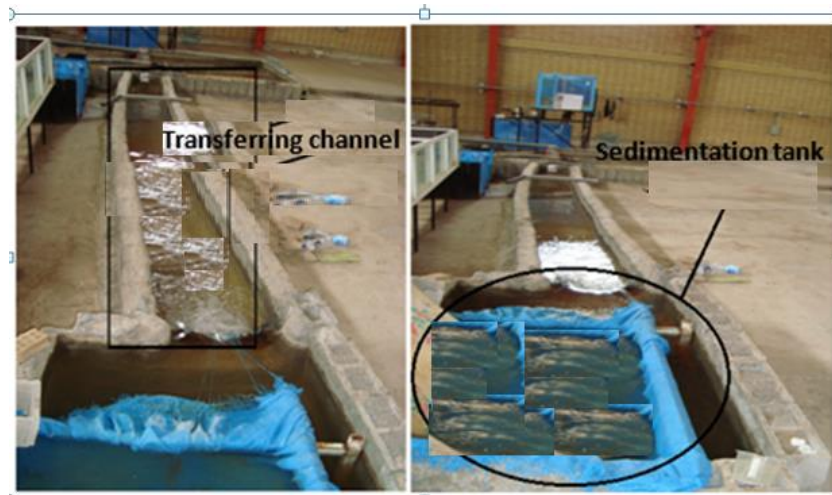
Figure 5. Schema of the sedimentation tank downstream to the lateral intake and transferring channel.
