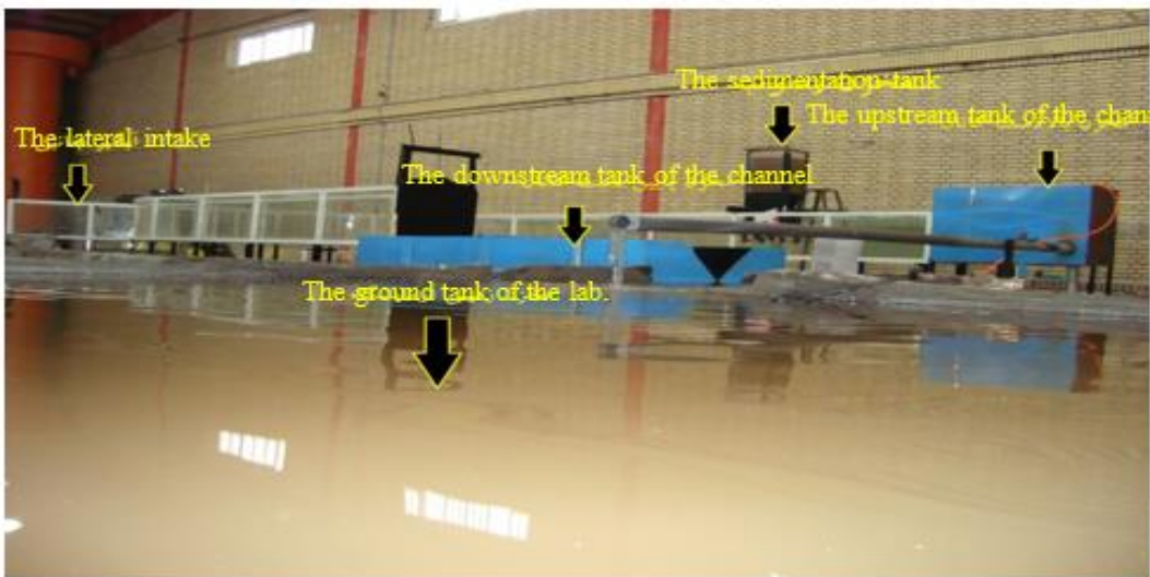
Figure 4. Schema of the laboratory flume and related equipment.
