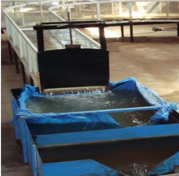
Figure 2. The sliding inlet for setting up the flow height.
