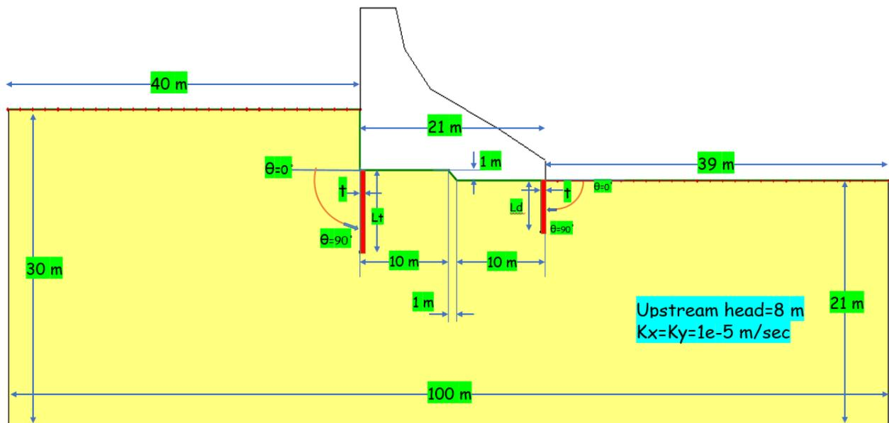
Figure 2. Schematic Cross-Section of the Cut-off Wall.
