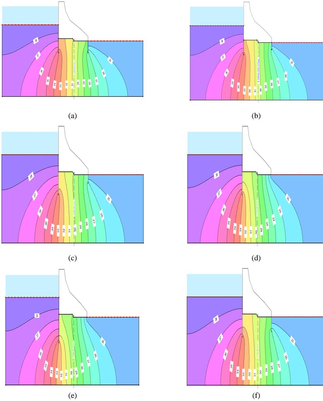
**Figure 4.** a) Contour lines for scenario Lt6 Ld3, b) Contour lines for scenario Lt6 Ld5, c) Contour lines for scenario Lt8 Ld0, d) Contour lines for scenario Lt8 Ld3, e) Contour lines for scenario Lt8 Ld5, f) Contour lines for scenario Lt10 Ld0, g) Contour lines for scenario Lt10 Ld3, h) Contour lines for scenario Lt10 Ld5.
