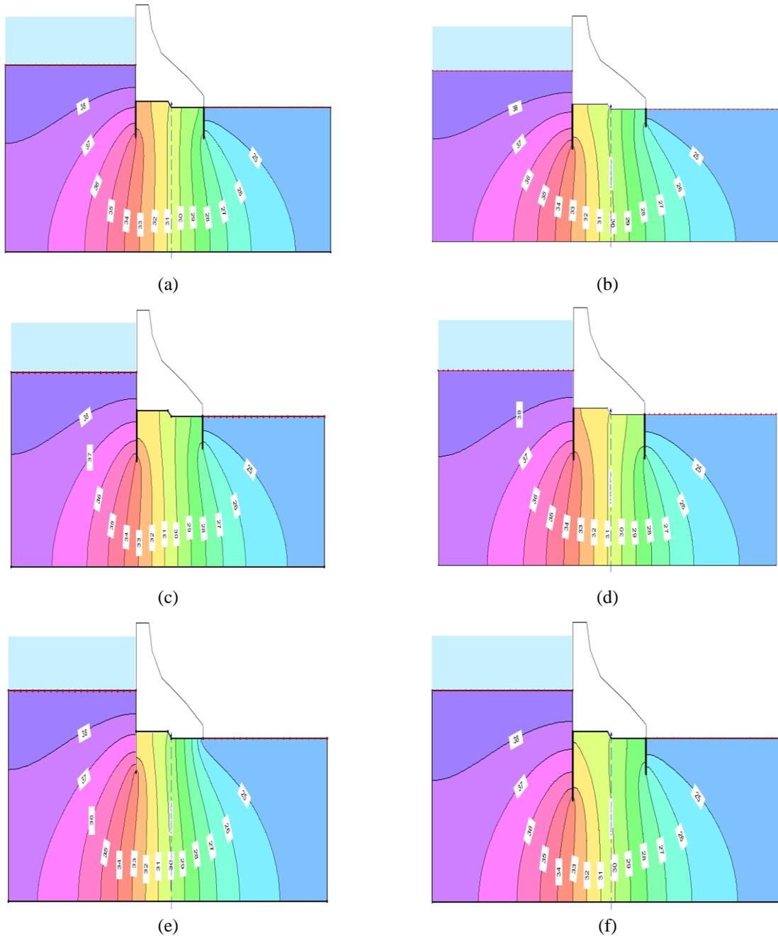
**Figure 3.** a) Contour lines for scenario Lt6 Ld5, b) Contour lines for scenario Lt8 Ld3, c) Contour lines for scenario Lt8 Ld5, d) Contour lines for scenario Lt8 Ld7, e) Contour lines for scenario Lt10 Ld5, f) Contour lines for scenario Lt6 Ld0.
