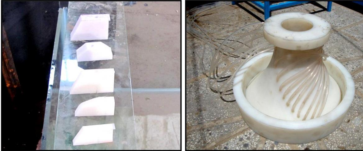
a. Different types of vortex breakers of Shaft spillway      b. installation manometer on the body of spillway
