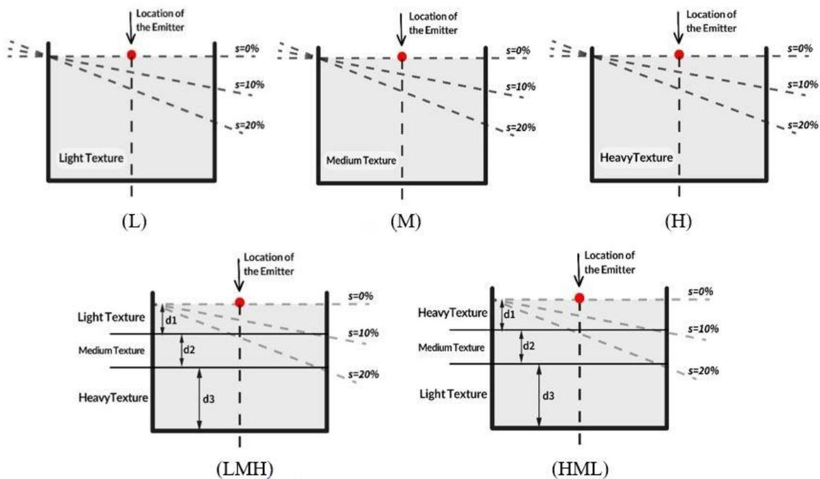
**Figure 2.** The schematic design of the experiments in this research.
