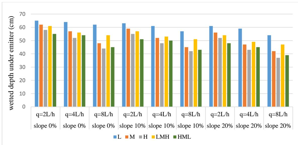
Figure 4. The wetted depths under the emitter in the five studied groups after irrigation
