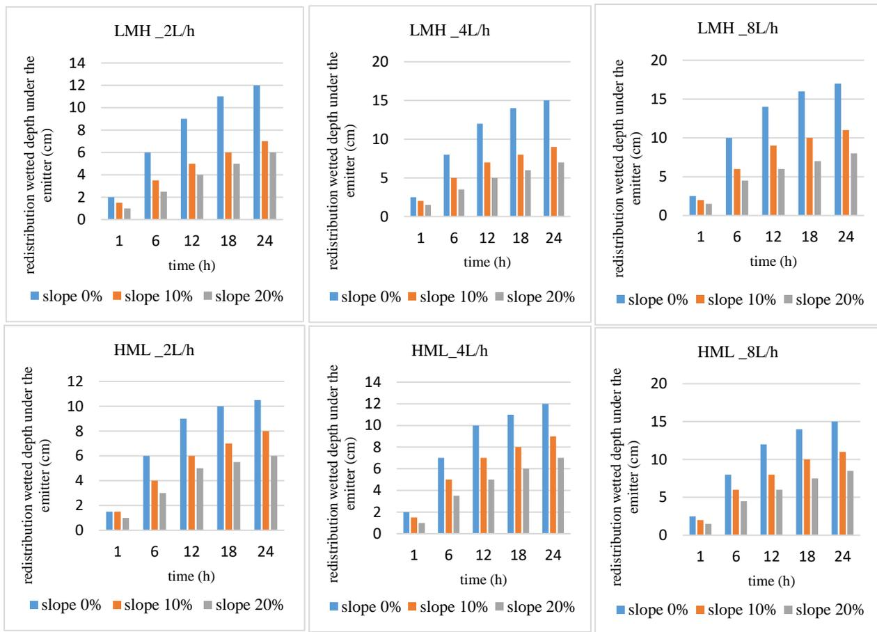
Figure 8. Wetted depth under the emitter after irrigation in the non-homogeneous soils
