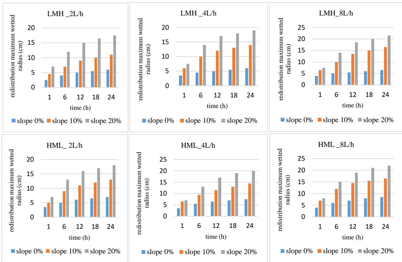
**Figure 6.** Maximum wetted radius after irrigation in non-homogeneous soils.
