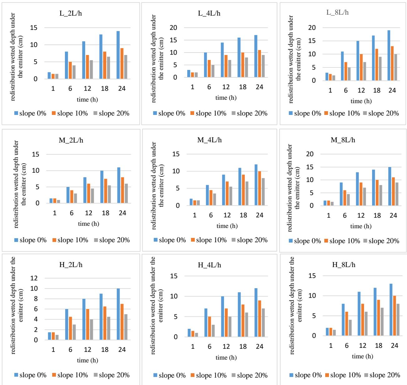
Figure 7. Wetted depth under the emitter after irrigation in the homogeneous soils.
